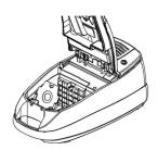
The dust cover will not close without a bag in the unit or if the bag is not inserted properly.
