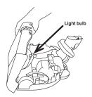
Simply pull the bulb out (no twisting) and reinsert a factory-authorized bulb. Place the top cover back on the unit, turn the machine over and re-insert the two top cover screws. Reinstall the bottom plate.
