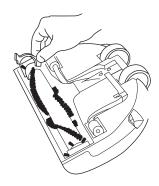
To reinstall the brushroll, reinsert the brushroll back into the unit (make sure the belt is attached properly). Next, insert the belt cover guard. Then, place the metal bottom plate back onto the unit (insert the front end of the bottom plate first). Re-insert the two bottom plate screws and secure.
