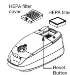
**NOTE:** Change the HEPA filter when the "service filter" light is illuminated on the power handle. Genuine HEPA filters cannot be washed or re-used.
