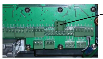
This view shows the removable connectors on the back of the master printed circuit board.
