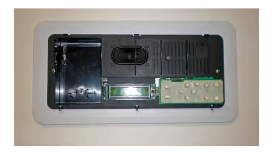
• Finish the master assembly by attaching the outer face plate and tightening the 3 screws on the bottom of the face plate.
